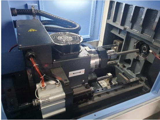
CONVERTIBLE TO NON GUIDE BUS H TYPE SPINDLE(BUILT IN MOTOR)
