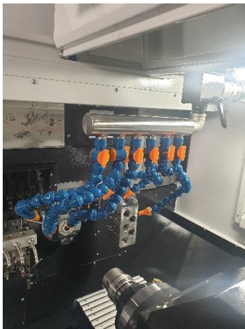
COOLANT PIPING NOZ ZLE
